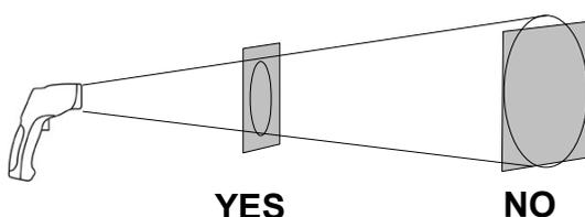
Make sure that the target is larger than the size of the laser sighting.
